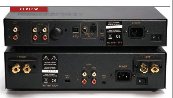
The HD120 offers a built-in 24/192 DAC, allowing access via USB, Bluetooth, coaxial, or optical input. A Burr Brown PCM 5102 DAC is well implemented here, and personally, I'd much rather see an excellent 24/192 DAC than a mediocre DSD DAC. Those of you with 12 DSD albums will need to look elsewhere.
